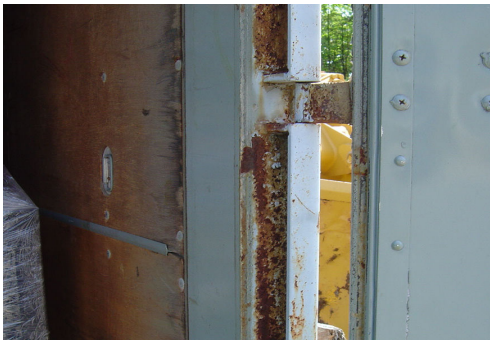
The storage container corrodes but not the equipment inside Intercept packaging.
